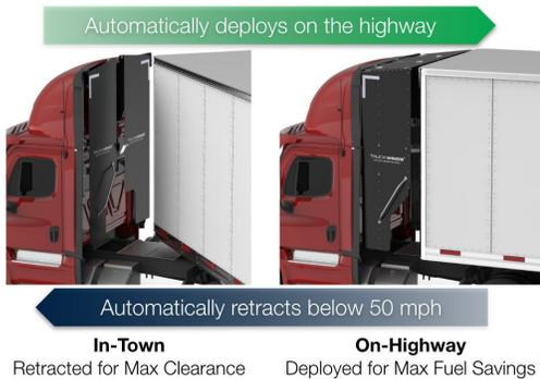
To address this challenge, Ryder evaluated TruckWings, an active aerodynamic device made by TruckLabs. TruckWings automatically deploys and closes the gap between the cab and trailer to reduce drag, improve handling, and save fuel. Improved fuel efficiency also means lower greenhouse gas emissions.
